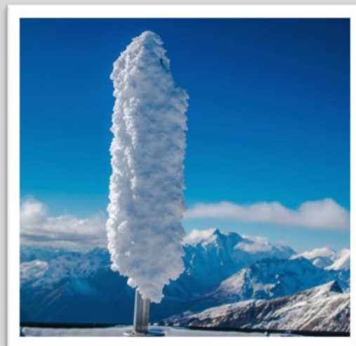
Abb.2: Eislastmessung am IceMonitor™. Fig.2: Iceload measurements with IceMonitor™. Quelle/Source: ZAMG/Hermann Scheer
