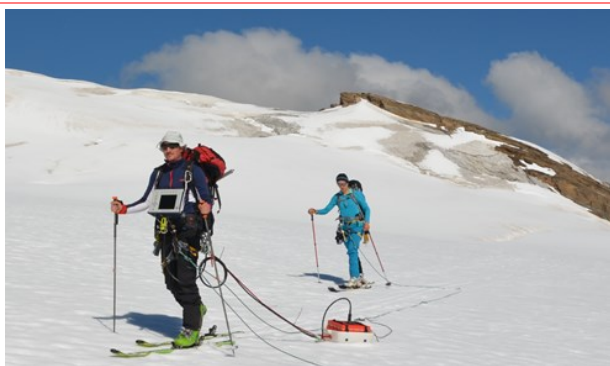
Abb.1: Akkumulationsmessung auf der Pasterze Fig.1: Accumulation measurements using ground penetrating radar Quelle/Source: ZAMG/G.Weys
