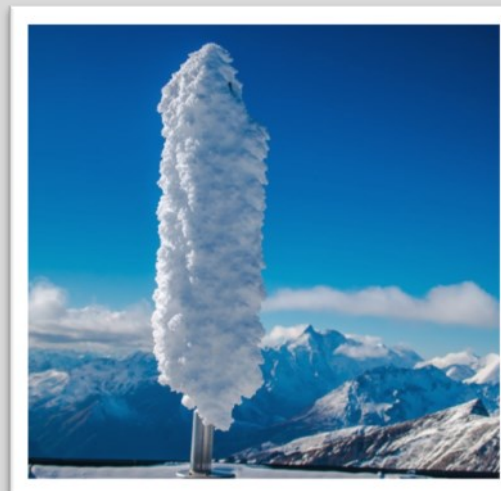
Abb.2: Eislastmessung am IceMonitor™. Fig.2: Iceload measurements with IceMonitor™. Quelle/Source: ZAMG/Hermann Scheer
