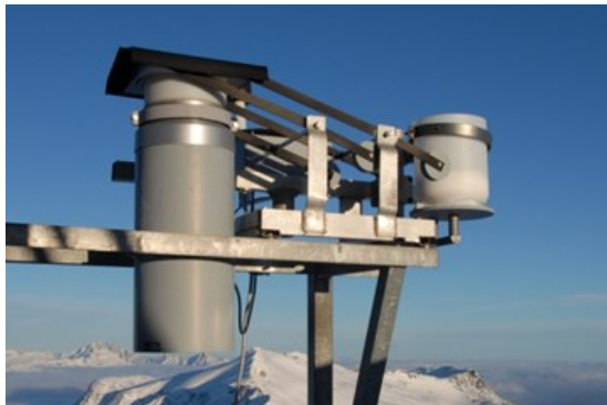
Abb.1: Sammler zur Schnee Probenahme - WADOS (Wet And Dry Only Sampler) Fig.1: Sampling of Snow with a WADOS (Wet And Dry Only Sampler) Quelle/Source: G. Schauer
