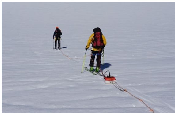
Abb.1: Akkumulationsmessung mittels Bodenradar Fig.1: Accumulation measurements using ground penetrating radar Quelle/Source: A. Neureiter
