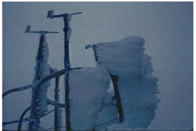
Heavy rime accumulation on the top of the tower. Note that the Pitot (on the far left) is free of ice (source MWO Archives)
