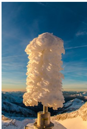
Eislastmessung am Sonnblick Ice load measurements at Sonnblick Quelle/Source: H. Scheer
