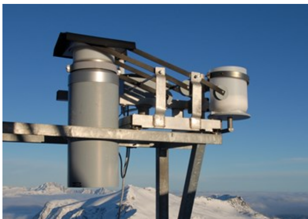
WADOS – Wet and Dry Only Sampler Quelle/Source: G. Schauer
