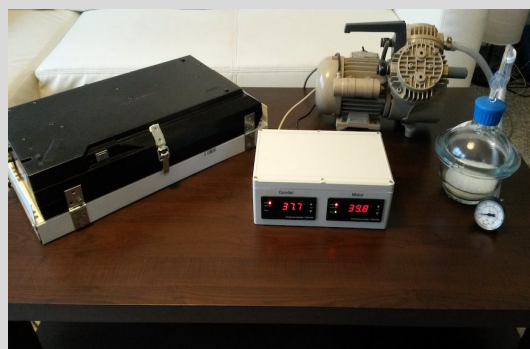
Kristallisation: Scanner links, Mitte: Temperaturmanagement, rechts: Exsikkator mit Manometer und hinten rechts: Vakuumpumpe Kristallisation: Scanner on the left, temperaturemanagement in the center, desiccator with manometer on the right and vacuum pump in the back
