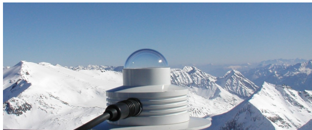
Abbildung 1: UV-Biometer zur Messung der erythem-wirksamen Strahlung. Figure 1: UV-biometer for measuring the erythemal radiation.
