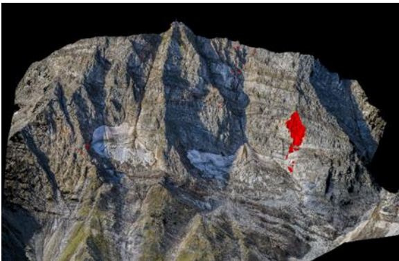
Abb.1: Felsstürze in der Nordwand des Hohen Sonnblicks 2021/2022 Fig.1: Rockfall source areas at the Sonnblick north-face 2020/2021 Quelle/Source: GEORESEARCH
