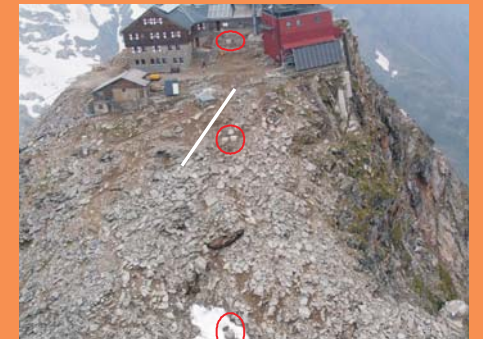
Fig. 9: meteorological observatory at Hoher Sonnblick, locations of geoelectric and drill holes
