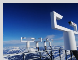
Abb. Particle Volume Monitor PVM | Fig.: Particle Volume Monitor PVM Quelle/Source: E. Ludewig, ACTRIS TC CIS
