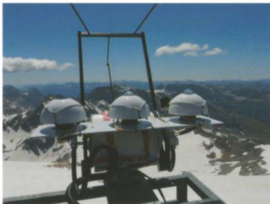
Illus. 1: Measuring instrument for recording percentages of direct and scattered, i.e. diffuse, solar radiation (Photo: Niedermoser)
