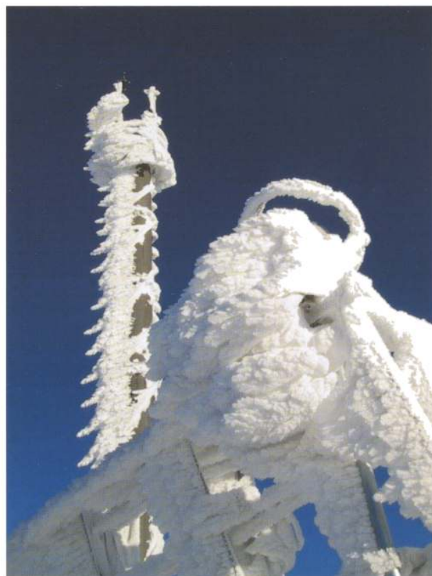
Illus.3: Wind measurement tower and global radiation unit following a night of white frost (Photo: H. Lindler)
