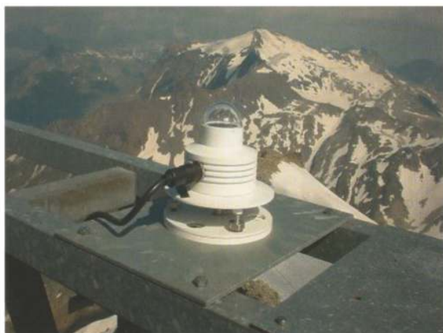
UV-Biometer at Hoher Sonnblick station, used to measure erythemally effective UV radiation
