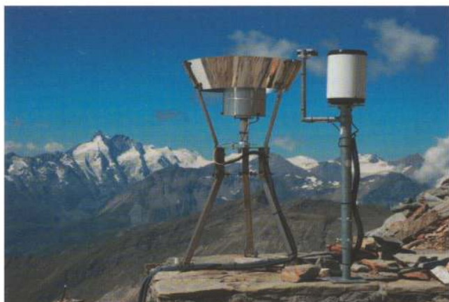
illus. 2: Precipitation measurement instruments on the south flank (Photo: W. Schöner)
