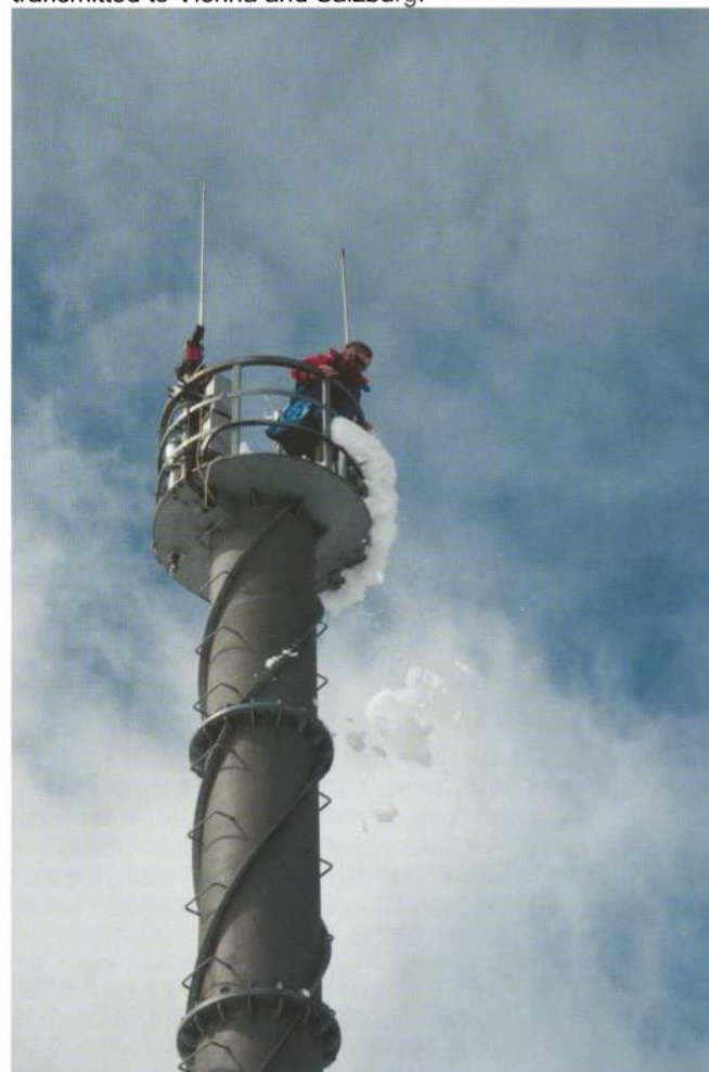
illus. 3: New wind tower with sonographic wind measurement (Photo: G. Weyss)
