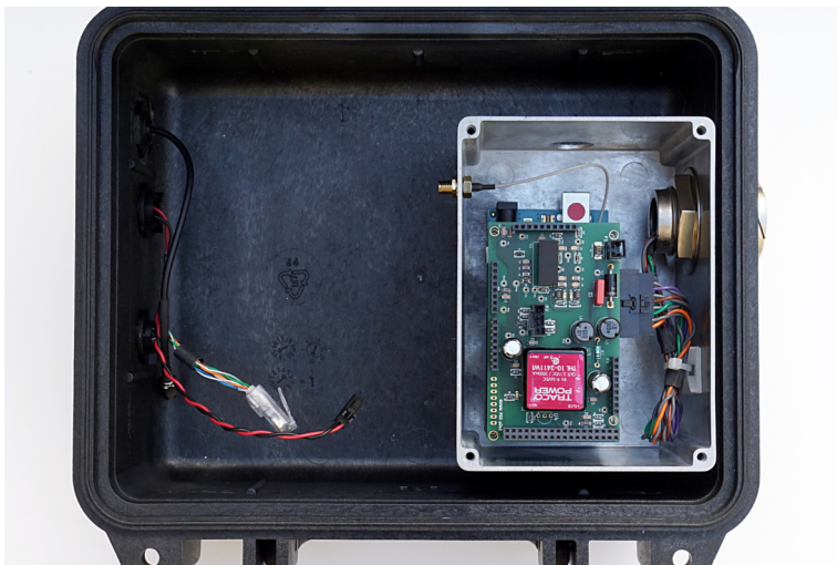
Figure 37: Put the analog sensor input cable with the pin cage in the Bulgin 7000 connector and connect the C-Grid connector on the Arduino stack. Fix the cable to the box using an adhesive base and a cable tie. If the position of the adhesive base is already known it's easier to mount the adhesive base and to fix the cable if the Arduino stack has not been put onto the Arduino.
