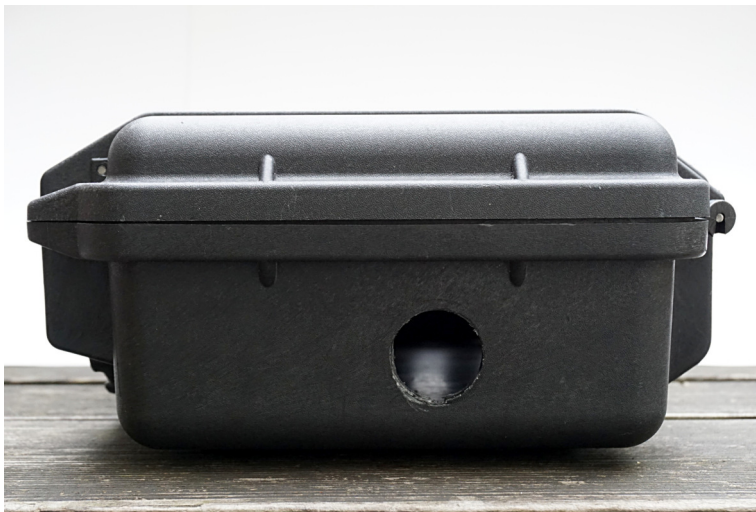
Figure 29: The drilled hole for the analog connector.
