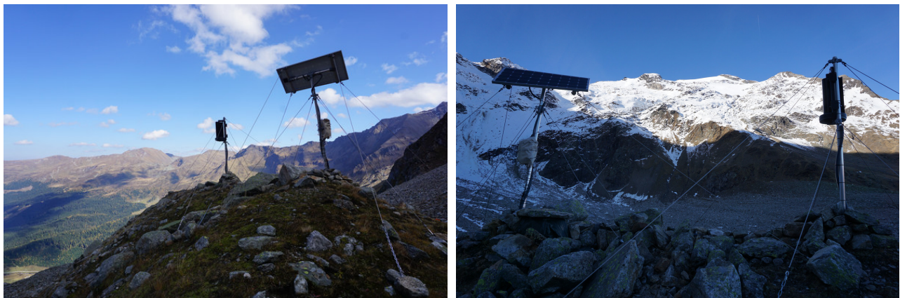
Figure 3.35: The mast and the solar panel were each stabilized by four guy wires. In summer 2017, a wind turbine was installed. The MOR station exhibits the lowest solar irradiance of all stand-alone stations.
