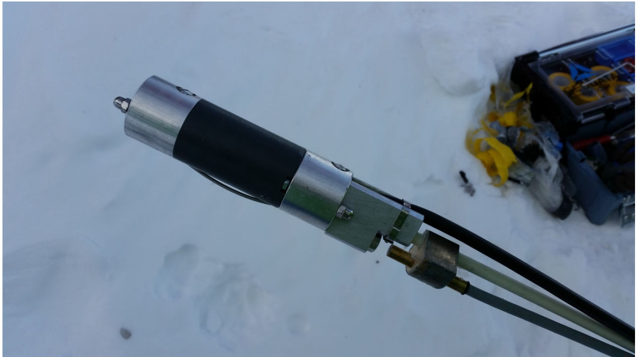
Figure 3.17: Geosono single component ( Z ) borehole sensor for the Kitzsteinhorn BH1 station. The sensor is mounted at the bottom of a stiff rod along which the thermistor string is also fixed.
