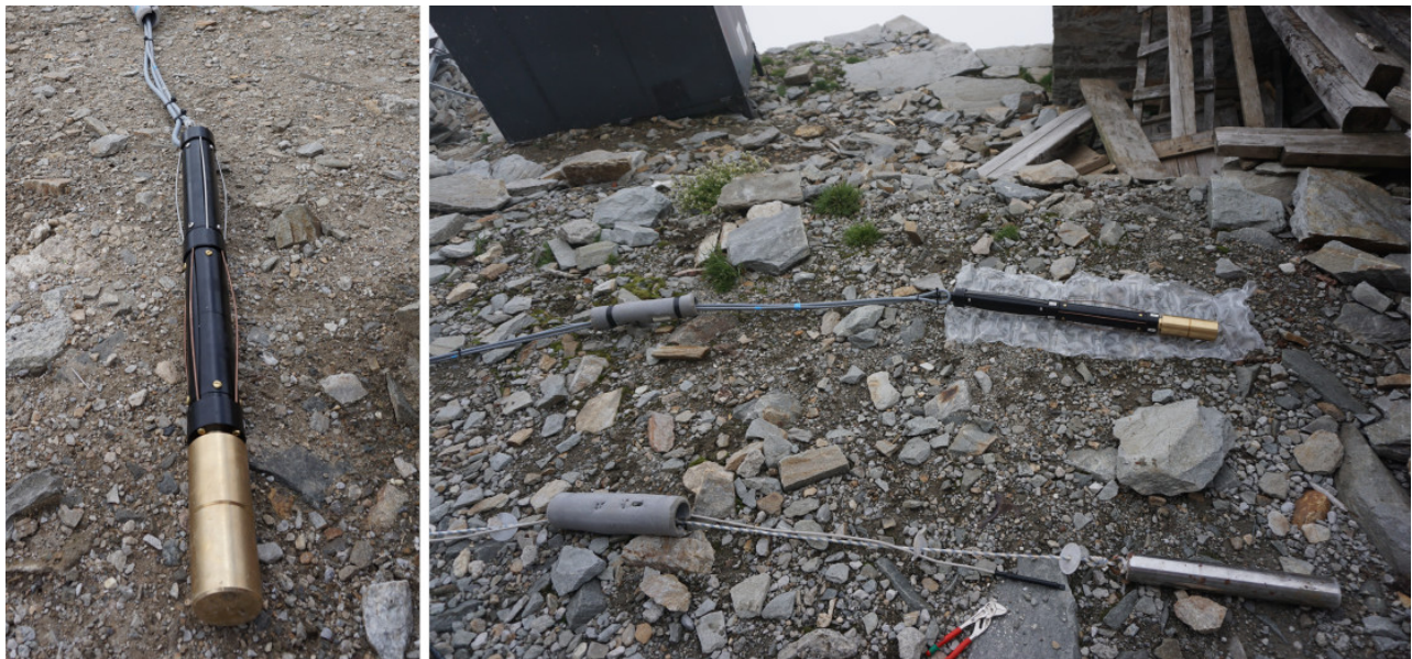
Figure 3.16: Three component ( X Y Z ) borehole sensor constructed by Geosono for the Sonnblick summit station (OBS). In the foreground of the right picture the thermistor string sinking weight is shown. The sinking weight was replaced by the seismometer.
