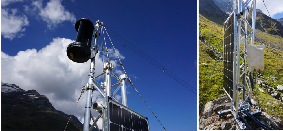
Figure 3.32: The new MIT station is equipped with a wind turbine. The Ruwai data recorder and the solar panel are mounted on a trussing element.
