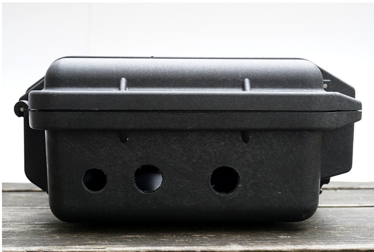
Figure 32: The drilled GPS, power supply and network connector holes.
