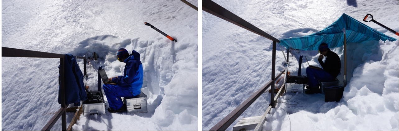
Figure 4.11: Several grounding strategies were tested to overcome the bad data quality of the Kitzsteinhorn network stations. Photos are taken during an extensive testing session at the BH1 station. However, all the efforts did not lead to better data quality, which left the Kitzsteinhorn unusable for further analysis.
