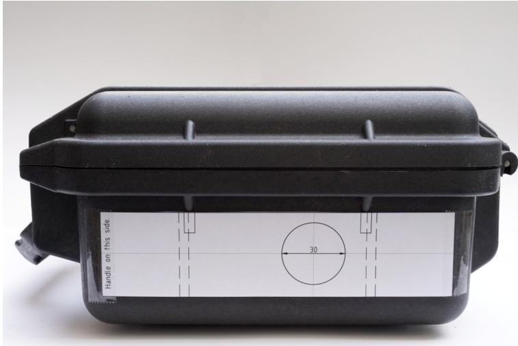
Figure 28: The pattern for the analog connector hole. Use a 30 mm holesaw for this hole. Align the pattern with the top fillets of the Peli case. Make sure, to place the pattern on the correct side. Use the handle bar of the Peli case as a reference.
