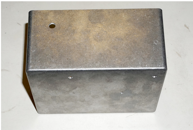
Figure 25: Use the same technique with placing the paper pattern on the box and marking the center of the hole for the GPS SMA connector hole. Use a 6,5 mm diameter drill for this hole.
