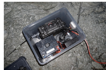
Figure 2: The unshielded Ruwai together with the power supply equipment in a plastic box.
