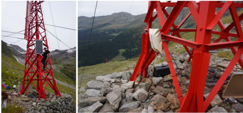
Figure 3.30: The first MIT station. The Ruwai data recorder and the solar panel were mounted on the SBO cable car pillar 'Mittelstütze'. The battery box was placed in the left corner of the basement's downward side.
