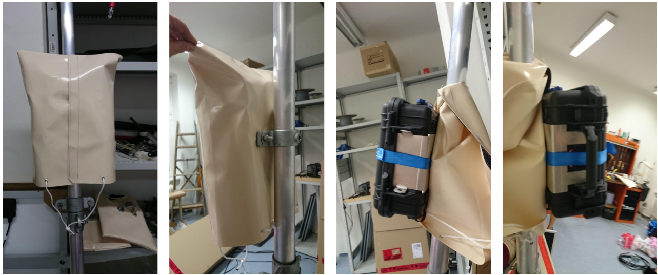
Figure 3.15: The Ruwai mast mount strategy. The core is the custom-built Pelicans 1200 aluminum mast mount. A tarpaulin cover provides additional protection.
