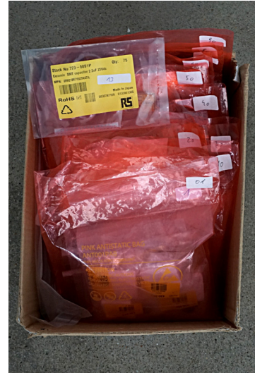
Figure 4: The organization of the electronic components using labeled plastic bags.
