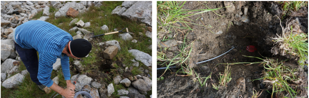
Figure 3.29: Geophones and cables were dug into the ground about 0.5 and 0.1 m, respectively, to suppress surface noise and potential damages by rockfall or wildlife.
