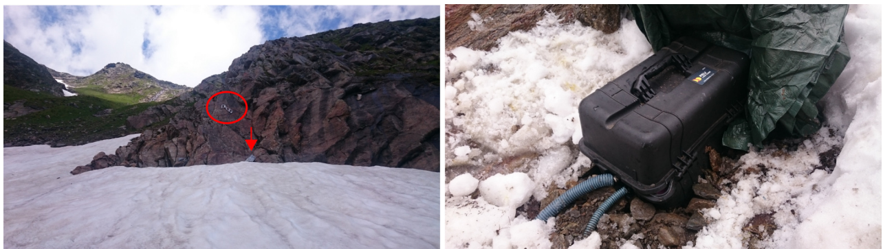
Figure 3.40: The left photo shows the solar panel remains after the winter season 2017/18. The remains of the solar panel frame are encircled in red, the arrow points at the crushed solar cells. The photo also illustrates PIL snow conditions on July 2, 2018. Furthermore, the huge snow load partly sheared off the lid of the battery box (right image).
