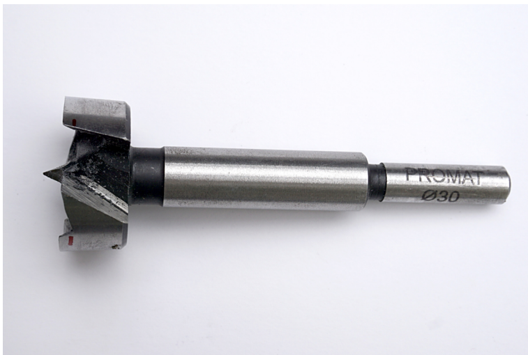
Figure 31: The GPS connector doesn't fit the wall thickness of 5mm of the Peli case. The wall thickness has to be reduced for this connector. First drill a small hole in the center of the GPS connector hole to transfer the center to the inside of the case. Then use a 30 mm diameter Forstner drill to create an inlay with a depth of ca. 2 mm on the inside of the Peli case to reduce the wall thickness to ca. 3 mm. I marked the needed depth on the drill using a permanent marker. Drilling this inlay from the inside was a little bit tricky. The Forstner drill mounted onto the drilling machine barely fit into the Peli case. Finally drill the hole using a 16 mm holesaw from the outside.
