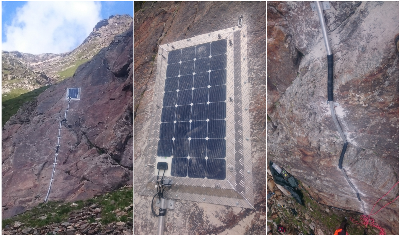
Figure 3.42: The new PIL solar panel installation. The GPS antenna is mounted at the lower left corner, next to the solar panel wiring.
