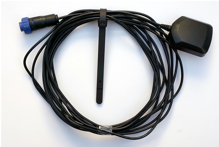
Figure 42: Assemble the Bulgin SMB cable connector to the GPS antenna which should be used together with the Ruwai data recorder.
