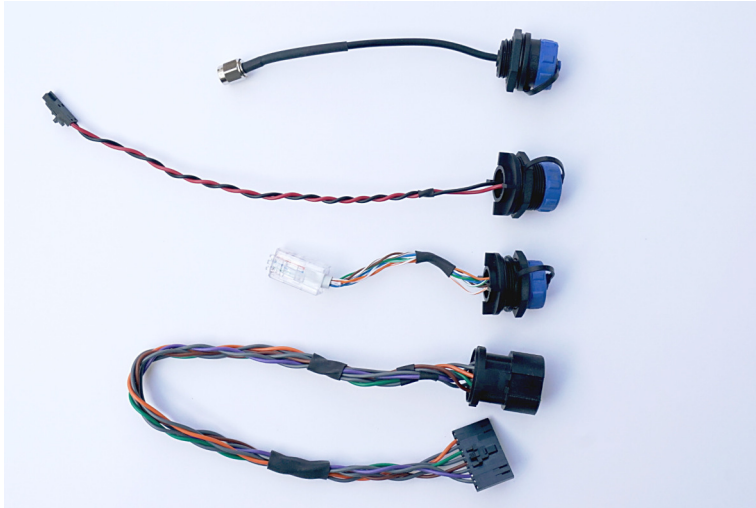
Figure 34: The connector cables from top to bottom: GPS, power supply, Ethernet and analog sensor connector.
