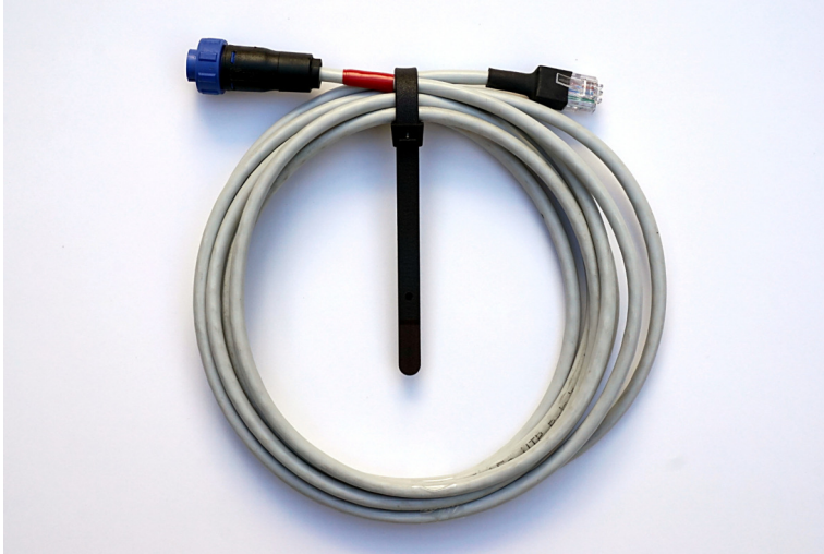
Figure 43: Assemble a crossed Ethernet cable if the Ruwai is connected directly to a computer or a straight Ethernet cable if the Ruwai is connected to a router or switch.
